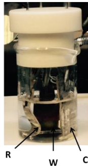
Figure C.1 3-electrode setup used for the electrochemical studies. Lithium pieces were used as counter and reference electrodes. Alligator type clips made with Titania were used as electrical contacts to decrease the resistivity that could arise from the contacts.
